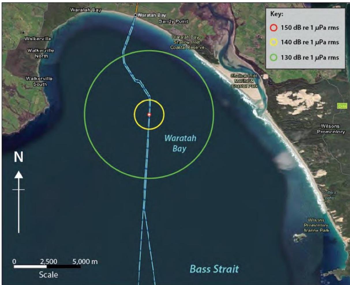
Notes: Blue dashed lines are the ML1 and ML2 bundled cables. White dot = cable ship and underwater noise source level. Coloured rings represent selected isopleths that can be shown at the scale of the map.
