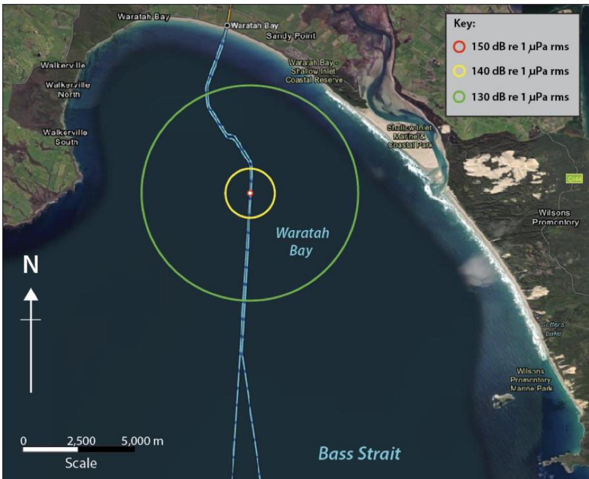
Notes: Blue dashed lines are the ML1 and ML2 bundled cables. White dot = cable lay ship and underwater noise source level. Coloured rings represent selected isopleths that can be shown at the scale of the map. Dashed blue lines denote the proposed alignments of the western and eastern monopoles of the project.
